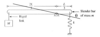
Let  $\theta$  be the clockwise angular displacement of the bar from the system's equilibrium position. Assuming small  $\theta$ , the potential energy of the system at an arbitrary instant is
