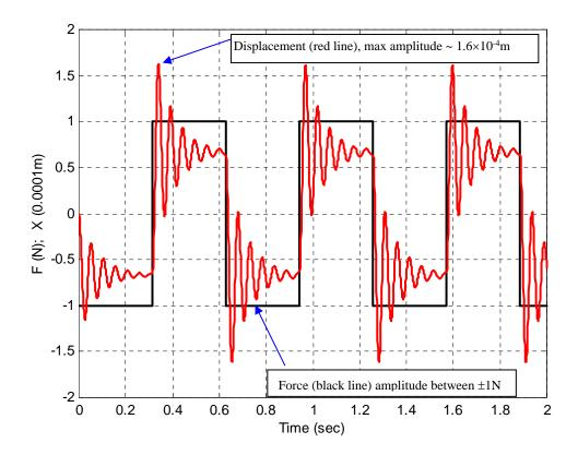
SOL: at steady state,  $F/x = K = 1/0.00006 \sim 1.67 \times 10^4 \text{ N/m}$ Estimated damped natural period  $\sim 0.21/4 = 0.0525 \text{ s} \rightarrow \text{damped natural}$  frequency  $\sim 120 \text{ rad/s}$
