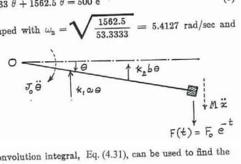
the forcing term as 500 e<sup>-t</sup>, the convolution integral, Eq. (4.31), can be used to find the steady state response as:
